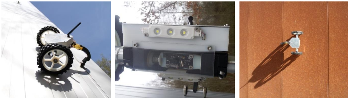
Fig. 3: The lightweight magnetic crawler. (source: DFKI GmbH)
